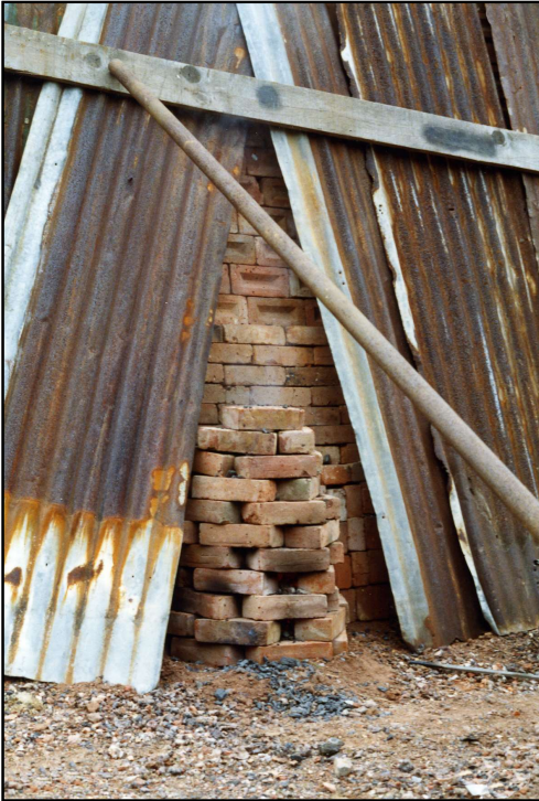
4.5. A small hole is left to fire the clamp. The wood fuel has already been built in as the clamp was built
