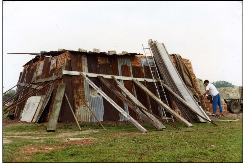
4.6. The finished clamp, covered in corrugated iron and lit, The temperature inside the clamp reaches 1500 C
