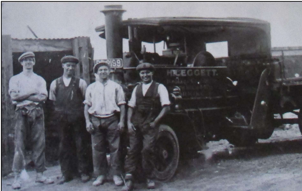
An early steam-powered lorry ready to be loaded with bricks at Bursledon Brickworks
