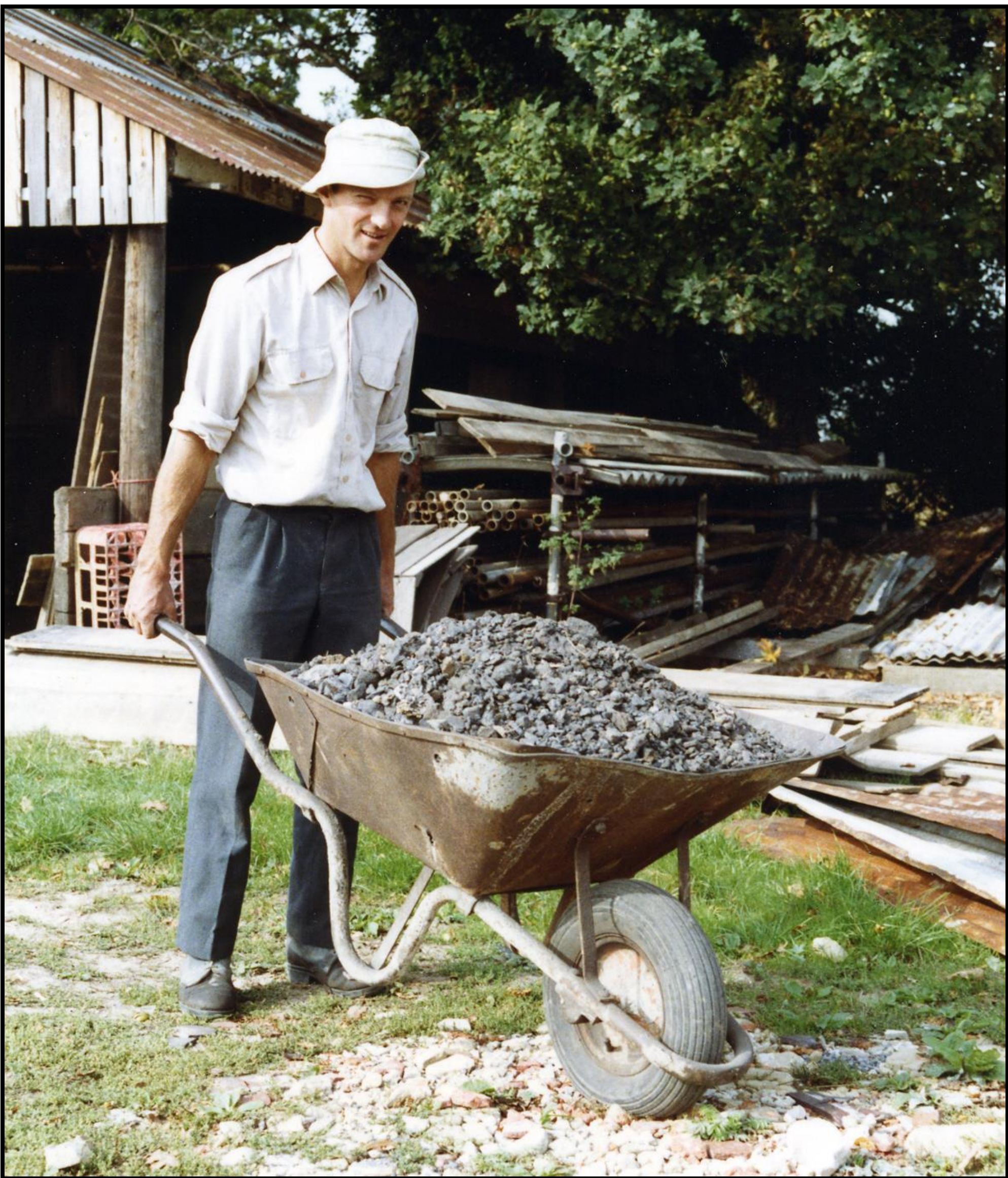
4.1. The bed of the clamp is prepared with a layer of ashes from previous firings
