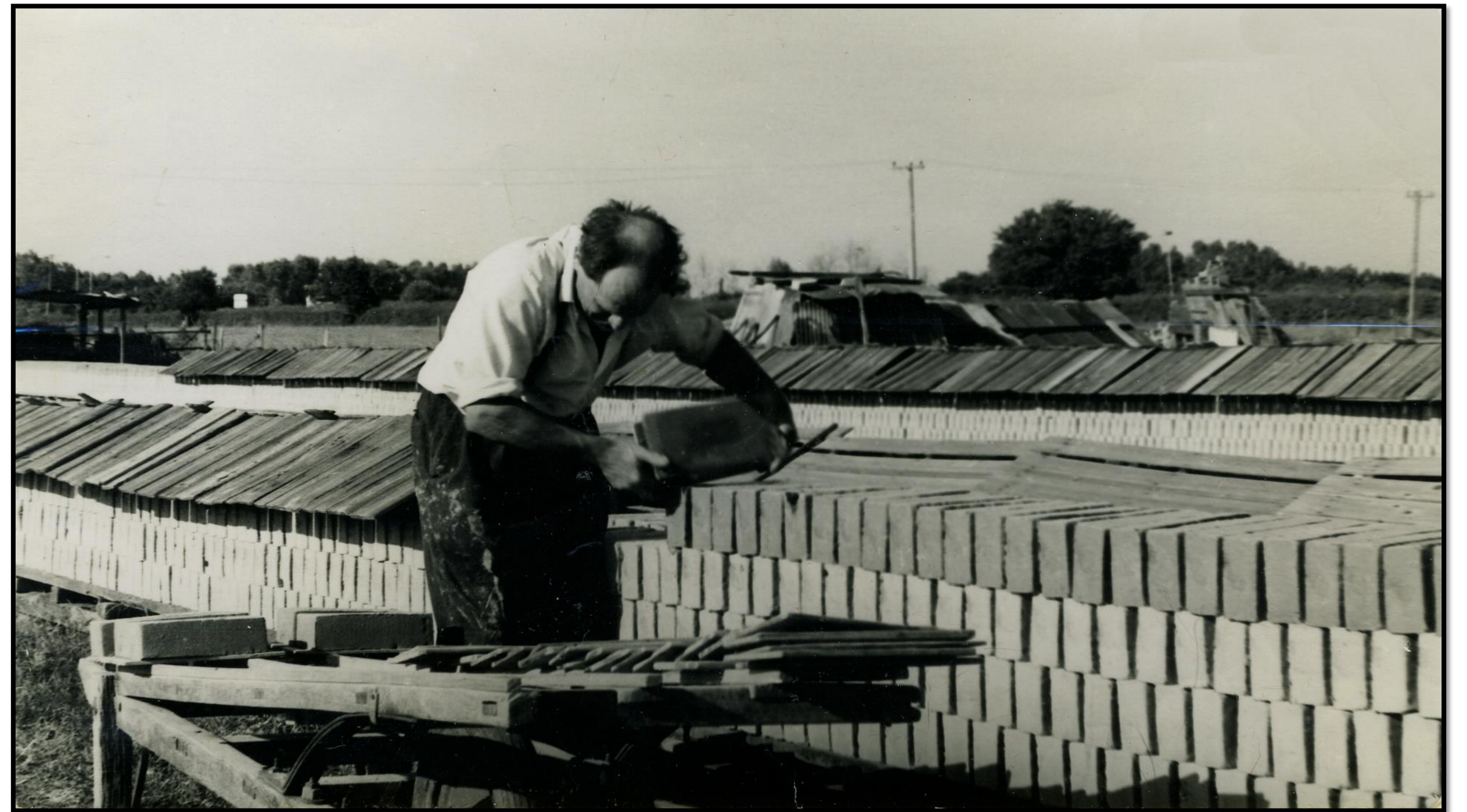
4.2. The newly made bricks are removed from the drying stacks to be built into a clamp.
